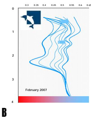
The traditional view has been ‘drying from top down’. In fact, drying typically takes place at a depth of around 2mtrs – for mature trees. The more direct the application of water to the drying zone, the quicker it will take effect.
