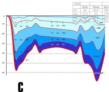
‘By month’ data (Figure D) has allowed us to correlate ground movement with changes in temperature and SMD values to assist in understanding which components exert the greatest influence (Figure C).
